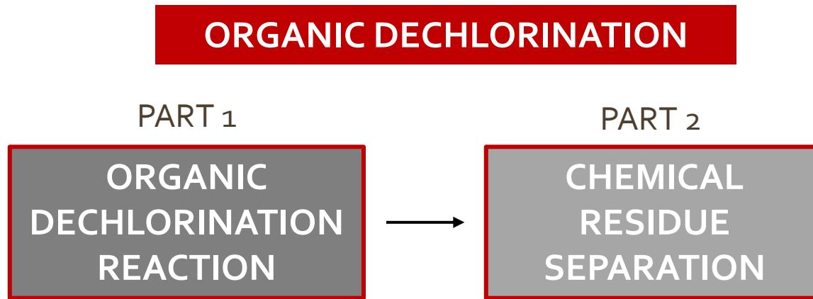
If **ORGANIC DECHLORINATION** is installed downstream PTU a single or double washing stage is needed to remove any traces of dechlorination chemicals together with chlorine residue.
